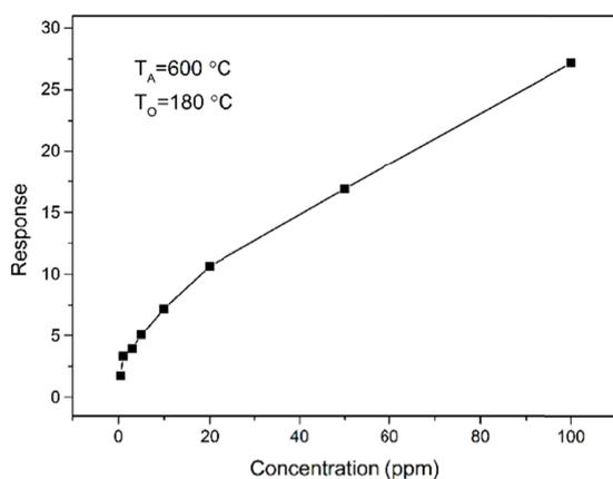
**Figure 3:** The response dependence on the acetone concentration for SnO<sub>2</sub> powders at the operating temperature of 180 °C.
