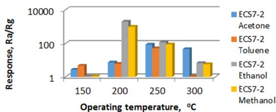
**Figure 6:** Comparison of ECS7-2 series sample responses to 1000 ppm different VOC exposure vs operating temperature.
