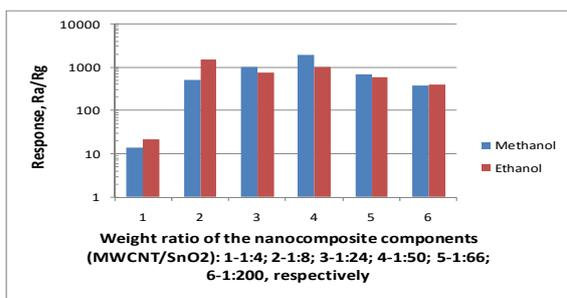
**Figure 5:** Response to 1000 ppm methanol and ethanol vapors at the operating temperature 200°C.
