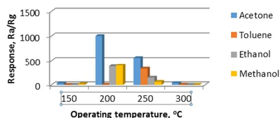
**Figure 8:** Measurements of the response (sensitivity) at different work temperature.
