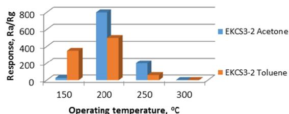
**Figure 7:** Response of EKCS3-2 set of samples to 500 ppm acetone and toluene vapors vs operating temperature.
