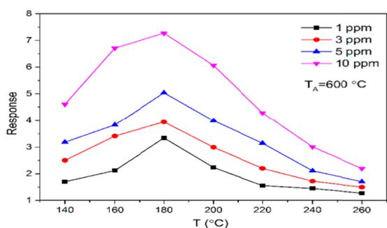
**Figure 2:** Response of sensors based on SnO<sub>2</sub> nanoparticles versus operating temperature to 1, 3, 5, and 10 ppm acetone, respectively.
