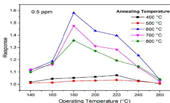
**Figure 1:** The response characteristics of the SnO<sub>2</sub> thick-films as a function of the operating temperature.
