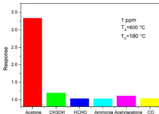
**Figure 4:** The response of the SnO<sub>2</sub> thick film to different gases with a concentration of 1 ppm at 180 °C.
