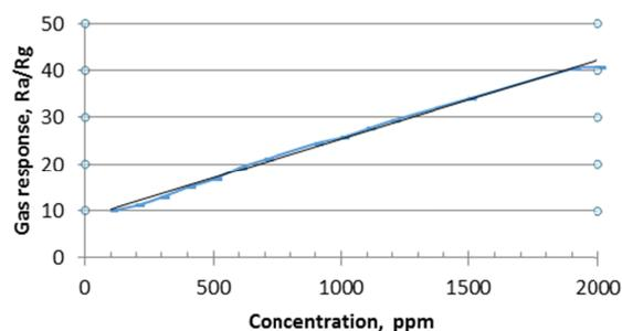
**Figure 9:** Dependence of the EKCS3-2 sensor response vs acetone vapor concentration.
