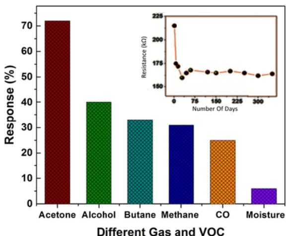
**Figure 11:** Selectivity study of the SnO<sub>2</sub>-0.25% MWCNT nanocomposite sensor measured at 250°C.
