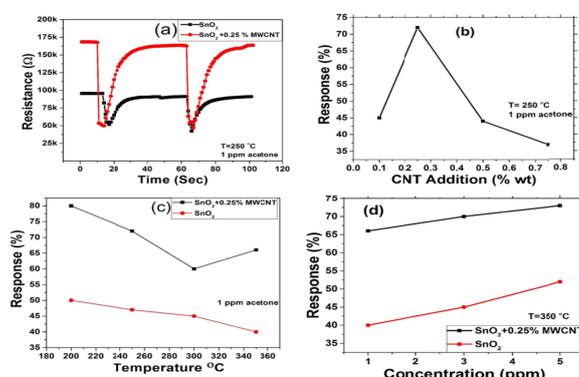
Figure 10: (a) Response of SnO<sub>2</sub> and SnO<sub>2</sub>-0.25% MWCNT sensors in 1 ppm acetone at 250°C. (b) Response of SnO<sub>2</sub> sensor in 1 ppm acetone for different CNT loadings at 250°C. (c) response of SnO<sub>2</sub> and SnO<sub>2</sub>-0.25% MWCNT nanocomposite sensors in 1 ppm acetone at different temperatures. (d) Response of SnO<sub>2</sub> and SnO<sub>2</sub>-0.25% MWCNT sensors in different concentrations of acetone at 350°C.
